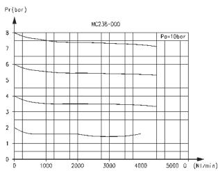
Pa = Inlet pressure (bar) Pr = Regulated pressure (bar) Q = Flow (Nl/min)
